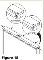
3. Remove the three screws located on the back of the handle (see **Figure 18**).
